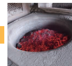
Dross taken out of the furnace
